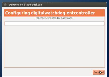
\* The password for the EC by default will be **blank**. If no new password is entered in the confirmation page, the new password will be **blank**.
